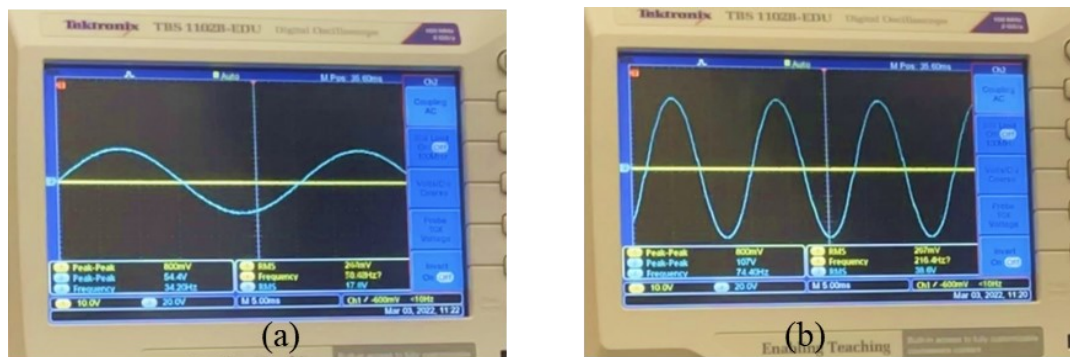
Figure 8. (a) Soft start; 40% voltage at 58 Hz (b) 100% voltage at 60 Hz
