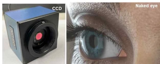
Fig 5. The method of image acquisition to detect colorimetric reaction: (left) CCD-based digital camera (right) the naked eye.
