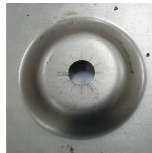
Fig. 10 Specimen after hole expansion test with cylindrical punch(DP980)
