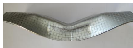
Fig. 11 Specimen after stretch flanging test with developed tool(DP980)
