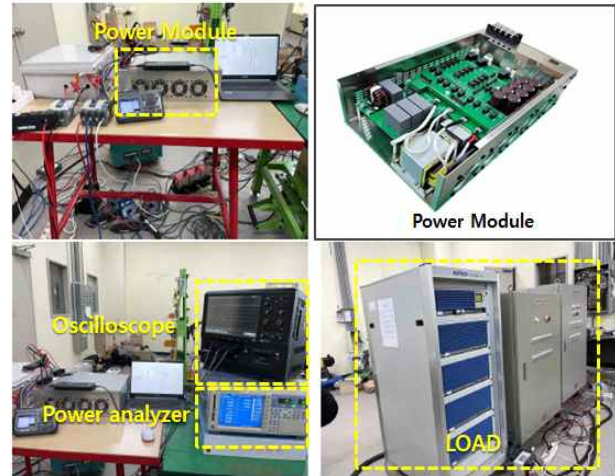
Fig. 6. Prototype of the proposed charger and rated test environment.
