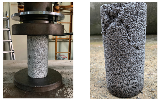
(a) Test setup (b) Failure pattern
