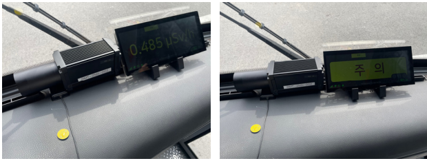
Fig. 9. Event using radiation check source (137Cs Disk source)
