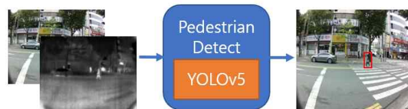
Fig. 3 The Structure of the Pedestrian Detector
