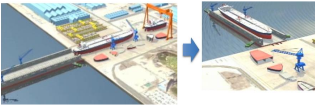
Fig. 3. Actual load-out method for on-ground build ship.
