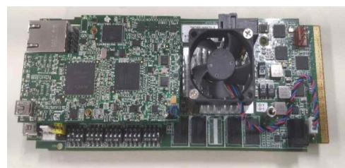
<Fig. 1> Photograph of the DSP evaluation board used to implement O-DU
