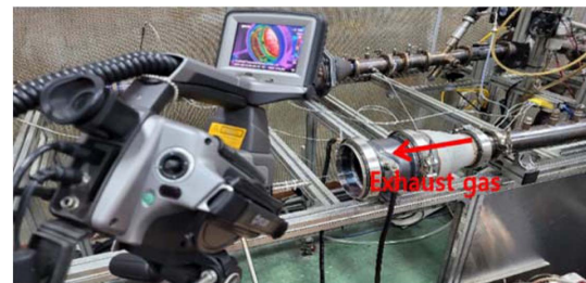
Fig. 4 Picture of setup for the measurement of heater surface temperature at EHC outlet using IR camera
