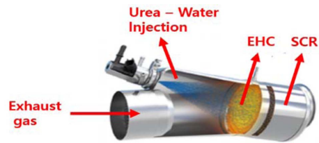
Fig. 1 Illustration of EHC-based urea-SCR system
