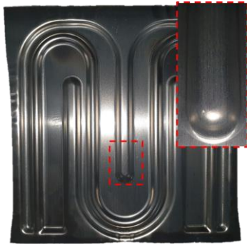
Fig. 14 Tryout result of heat exchanger separator using the crash forming
