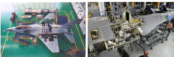
<Figure 1> F-16 Fighter in Depot Maintenance[32, 33]
