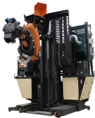
<Figure 3> Advanced Robotic Laser Coating Removal System
