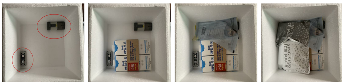
Fig. 2. Fresh foods and data logger in EPS cooling packaging box for delivery service.
