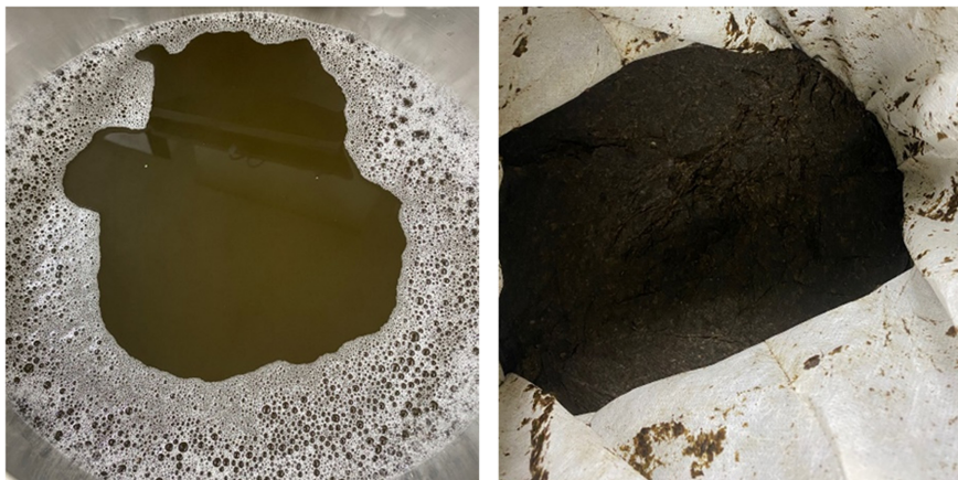
Fig. 5. Fermentable sugar and Residual solid obtained after dilute acid pre-treatment using a 30 L reactor (Left: Fermentable sugar, Right: Residual solids, reaction conditions: reaction temperature 121°C, reaction time 15 min, H 2 SO 4 concentration 1.0 wt. %, solid : liquid = 1 : 15).
