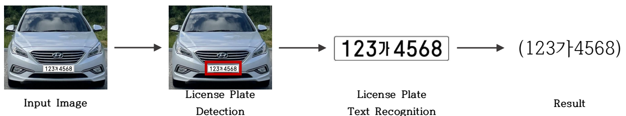
Fig. 1. Structure of Existing Car License Plate Recognition System
