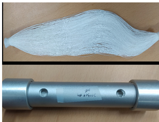
Fig. 1. Images of pristine PDMS hollow fiber membranes and module.
