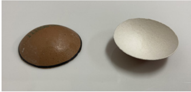
Fig. 6. Cutaway for measurement of shell electrical conductivity.
