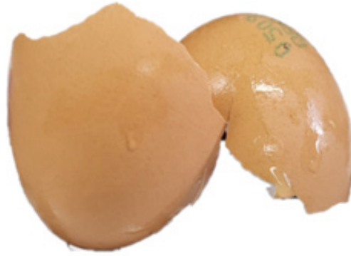
Fig. 5. Break point for shell thickness measurement.
