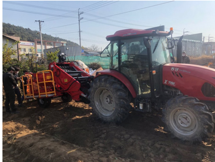
Fig. 1. A photo of agricultural tractor with underground crop harvester used in this study.
