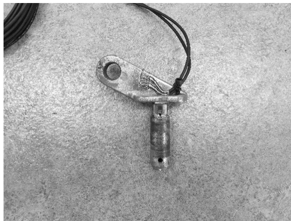
Fig. 5. A photo of machined eyebolt for measuring traction on eyebolts.
