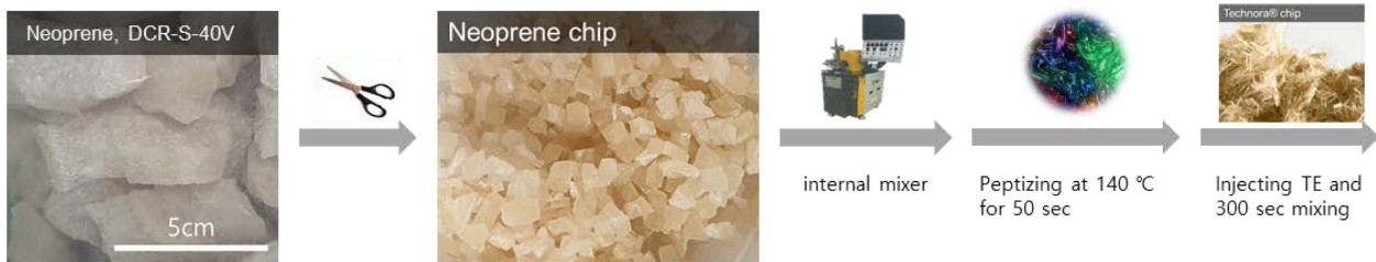
Scheme 1. Manufacturing Process of TE-NP composite using Internal Mixer.
