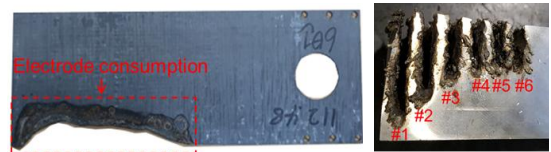
(a) Electrode consumption (b) Material removal Fig. 5 Electrode consumption and material removal after CAMC process
