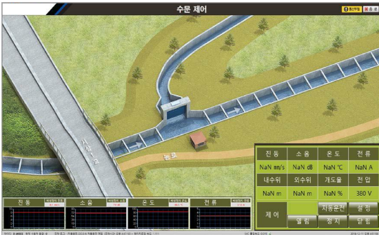
Fig. 7 Communication loss status program screen
