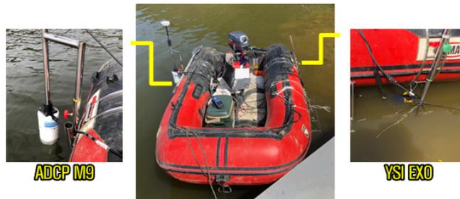
Fig. 2. Measuring Equipment ADCP, YSI-EXO
