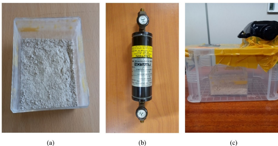
Fig. 3. (a) A tray containing monazite powder as thoron source, (b) a radon source of Pylon RN-1025 containing Ra-226, (c) a big box for mixing radon and thoron and a pump placed on the box.
