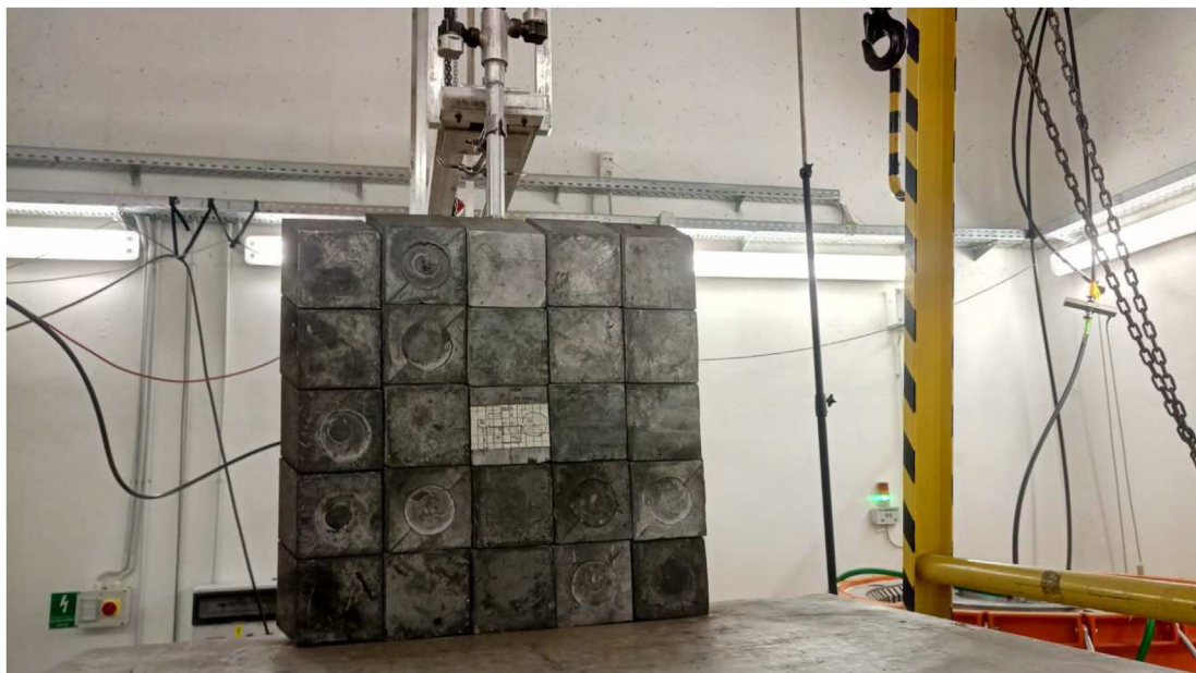
Fig. 2. Lead bricks configuration containing activation foils holder made of aluminium.
