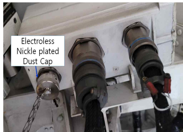
Fig. 21 Improved electroless nickel plated dust Cap installed to the aircraft
