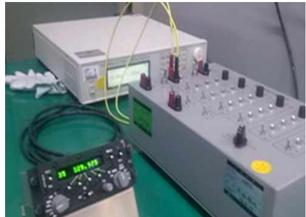
Fig. 5 Reproduction test of U/VHF radio and intercom reception noise
