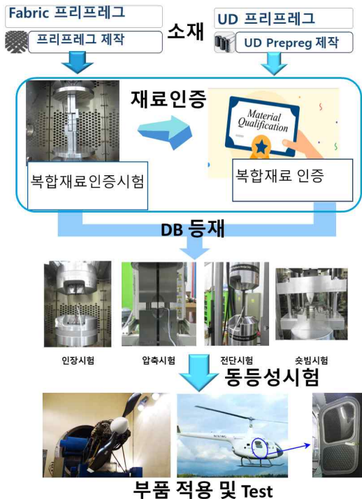
Fig. 7 Compliance Validation Process for Composite Part Manufacturing
