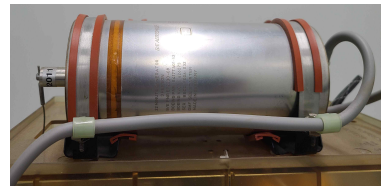
Fig. 8. Emergency oxygen generator (B777-200ER)
