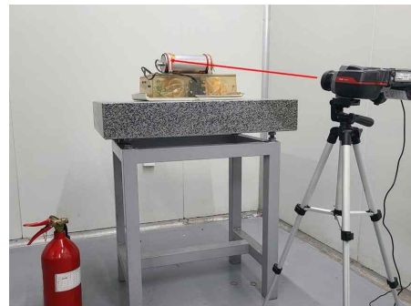
Fig. 9. Emergency oxygen generator operation test
