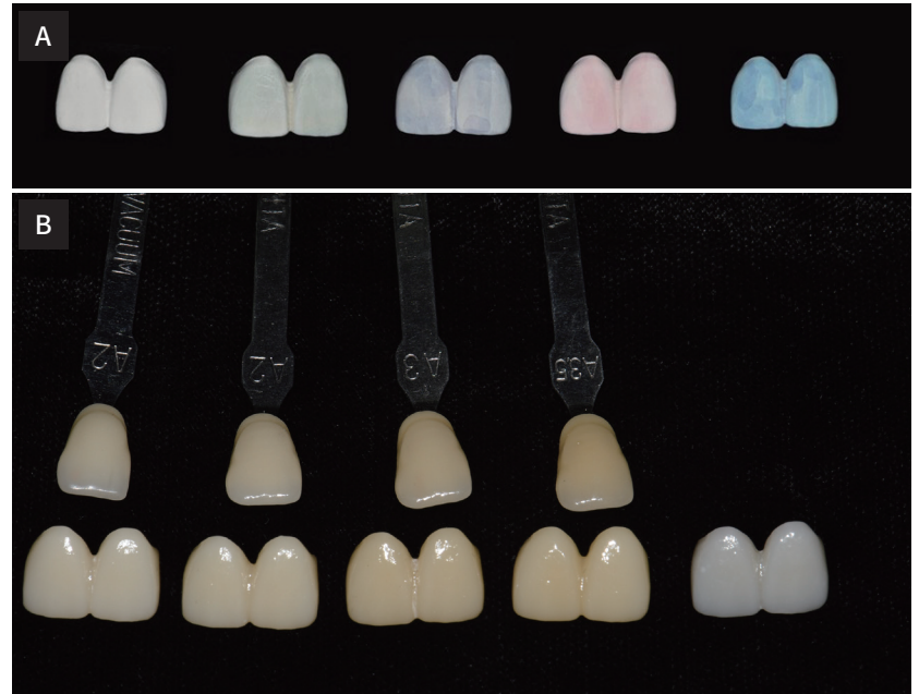
Fig. 2. (A) A2 Zirconia Block (Ceramil Zolid HT+PS) using various coloring liquids like Control, A2, A3, A3.5, Enamel, (B) Comparing of A2 zirconia block (Ceramil Zolid HT+PS) using various coloring liquids with VITA classical A1 - D4®.
