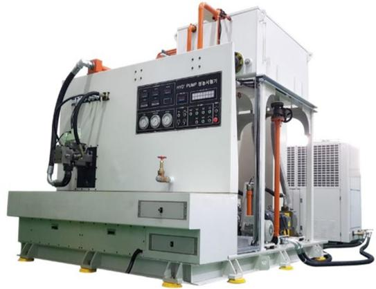
Fig. 11 Performance test bench of the piston pump
