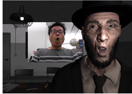
Fig. 2 The result of applying facial motion of a virtual human based on a real human: It can express virtual human's facial motion in real-time.
