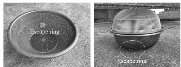
Fig. 1. Experimental basket for escape ring performance of giant octopus used in tank experiments.
