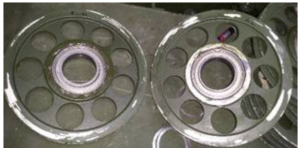
Figure 7. Interference between Pulleys
