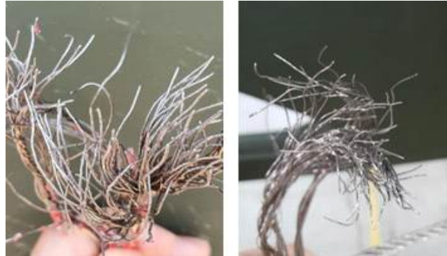
Figure 3. Propulsion Wire Fracture
