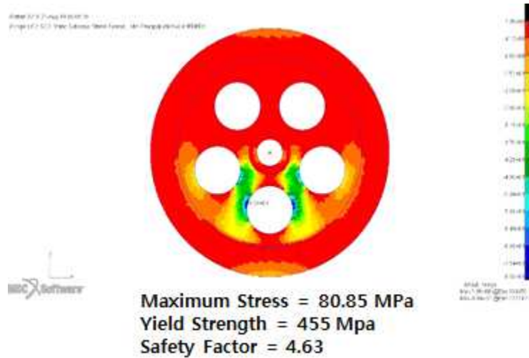
Figure 16. FEM Analysis Result(Modified Front Pulley)
