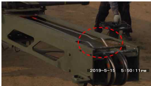
Figure 6. Abnormal Behavior of Propulsion Wire
