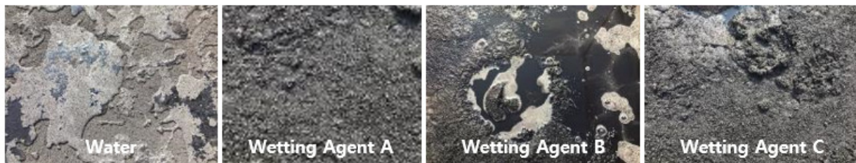
Fig. 2. Results of infiltration of wetting agents and fire water into the deep seated part of coal
