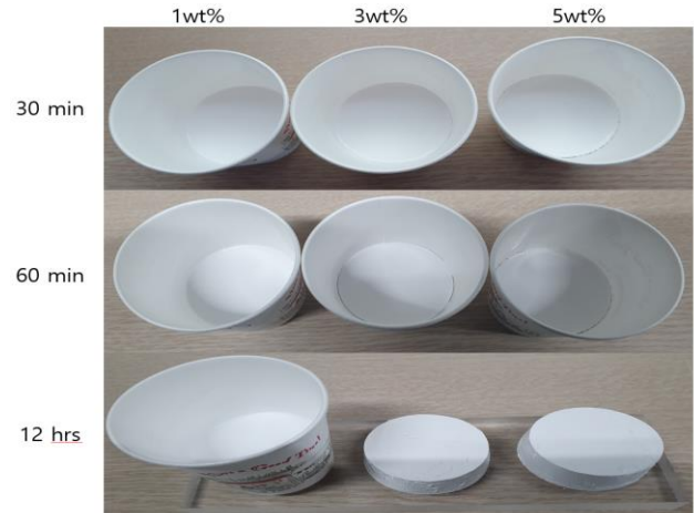
Fig. 7 Drying time change with monomer content
