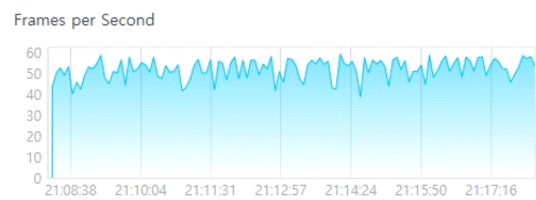
Fig. 8 FPS at 5,000 targets with H.265
