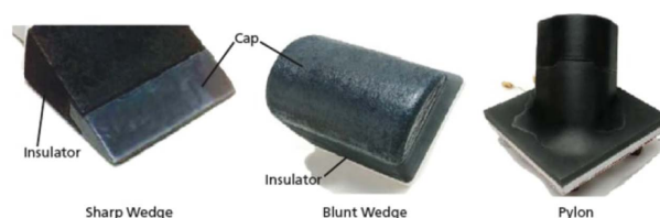
Fig. 4. Various configurations of TUFROC samples [21]
