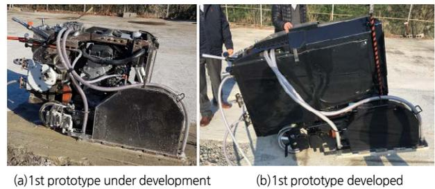
Fig. 8. Eco-friendly pavement cutter developed (Kim et al., 2019)
