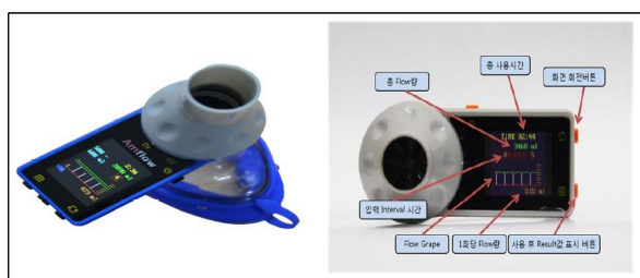
Fig. 3. The external appearance and measuring screen of flowmeter
