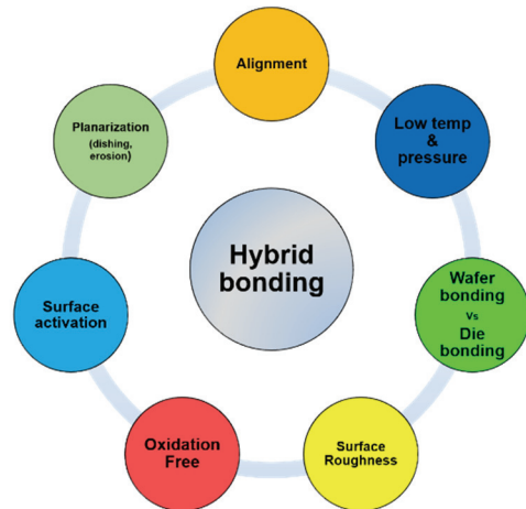
Fig. 6. Key factors to consider in hybrid bonding. 32)
