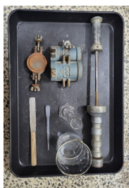
Fig. 4. Equipment for compaction tests
