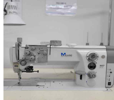
Figure 3. Sewing Machine with a Single Needle (taken by author)
