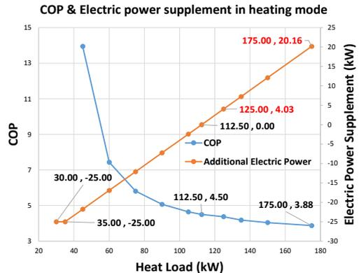
Fig. 5. Cogeneration system COP in heating mode
