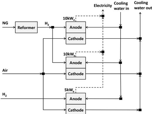
Fig. 3. Schematic diagram of 25 kW PEMFC system
