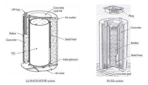
Fig. 5. Overviews of MAGNASTOR and concrete silo systems.
