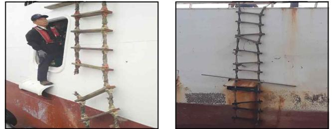
Fig. 6 Damaged pilot ladders (BHPA, 2023)
