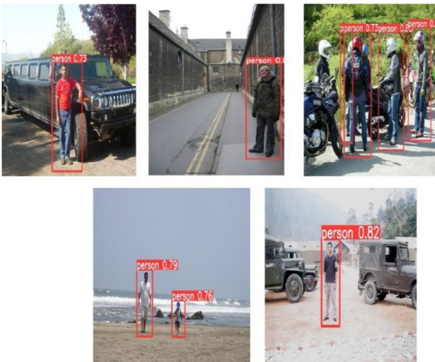
Fig. 9. Image examples of human detection test results of the YOLO model trained with semi-synthetic human data.
