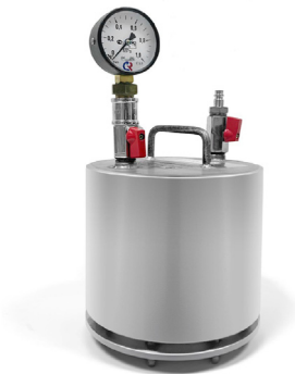
Fig. 2. Metal Marinelli vessel for the measurements of RNG activity concentration.
