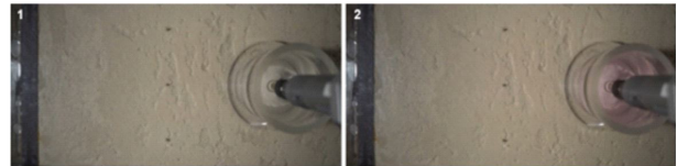
Fig. 7. Changes in the Riverbed during the Experiment for Case S2012 ( \Delta H/L=0.24 , d_{50}=0.16mm )
