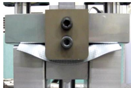
Fig. 9 Stretch flange test with straight shear line specimen
