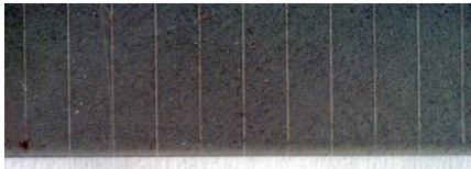
Fig. 5 Specimen laser-marked with evenly spaced stripes
