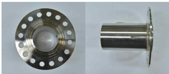
Fig. 7 Combustion Chamber for Ignition Test
